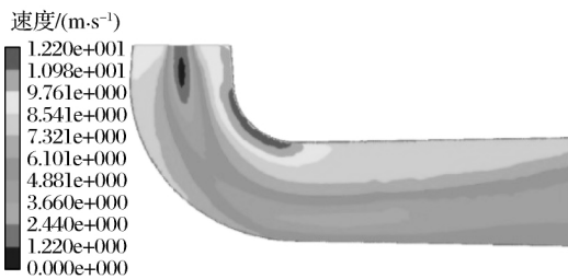
图 7 等截面无隔板尾水管速度分布(导叶开度 80%) Fig. 7 Velocity distribution in the prismatic draft tube without clapboard(gate opening 80%)
