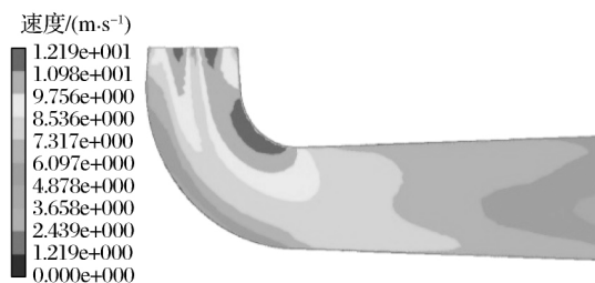
图 11 等截面无隔板尾水管速度分布(导叶开度 100%) Fig. 11 Velocity distribution in the prismatic draft tube without clapboard(gate opening 100%)
