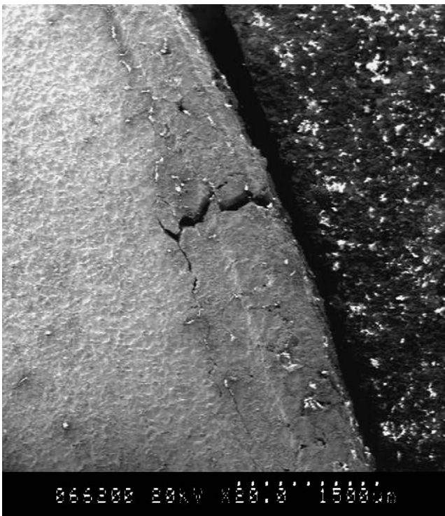
Fig. 10. Fracture SEM of the specimen with infiltrated layer at the bottom.
