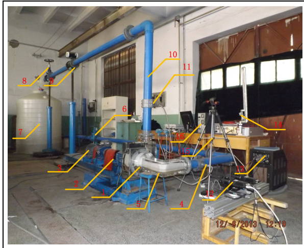
Figure 9. The open PIV test comprehensive experiment platform for the type of 100LN-32 screw centrifugal pump. 1: 150 × 100LN-7 transparent screw centrifugal pump; 2: torque meter; 3: electric motors; 4: inlet piezometer tube; 5: inlet conduit; 6: gate valve; 7: water storage tank; 8: manual control valve; 9: electromagnetic flowmeter; 10: outlet conduit; 11: outlet piezometer tube; 12: CCD camera; 13: generating laser; 14: laser head; 15: spider; 16: PIV image processing system.
