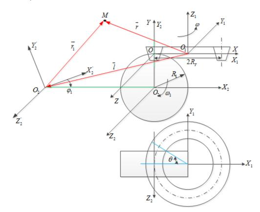
Fig. 1 Principle of forming a VH-CATT gear
