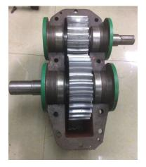
(a) (b) **Fig. 4** Manufacture of the VH-CATT gear sample
