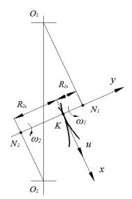
Fig. 5 The relationship between geometry and kinematics of the VH-CATT gear
