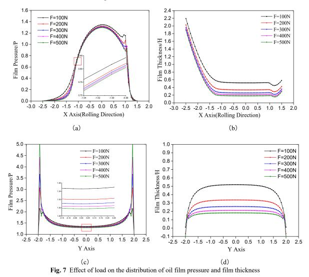
5.1 Effect of load on oil film pressure and oil film thickness
