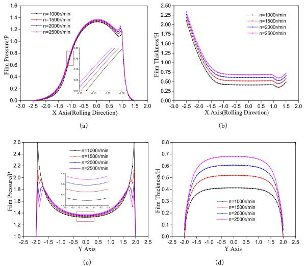
5.2 Effect of entrainment velocity on oil film pressure and oil film thickness
