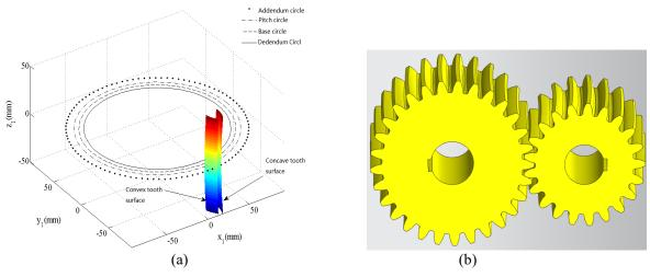
Fig. 2 Meshing model of the VH-CATT gear
