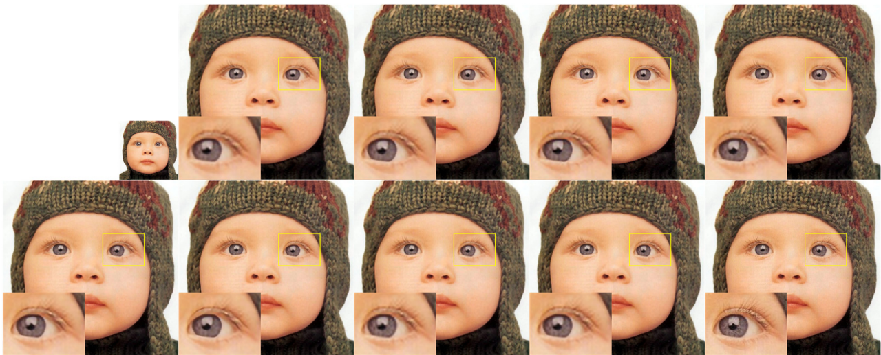
Fig. 6. SR results of the image ‘baby’ from Set5 for upscaling \times 3 . Images from top to bottom and left to right: LR input image, reconstructed HR image by Zeyde et al. [9], A + [21], SelfExSR [39], SRCNN [40], FSCNN [41], VDSR [42], our SCSR, and our proposed AMSRR-SCSR, as well as the ground truth HR image.
