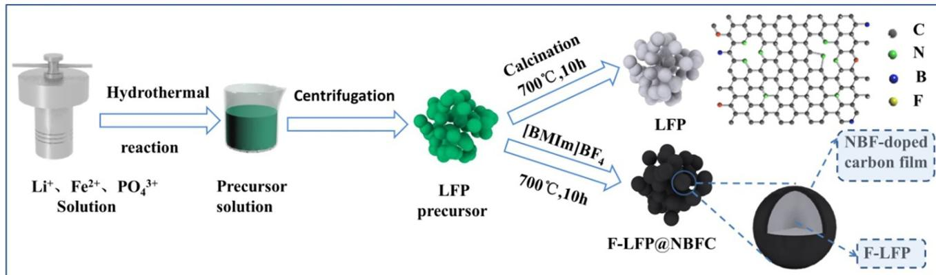
Fig. 1. An illustration of synthesizing F-LFP@NBFC.
