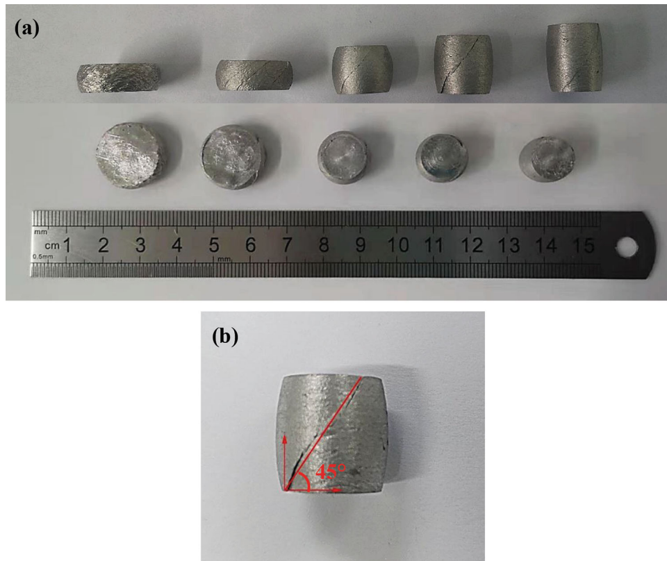
Fig. 9 Morphologies of as-cast compression specimens: (a) pure Al with various HEA addition (0, 5.0, 10.0, 15.0 and 20.0 wt.%); (b) AMCs adding 15.0 wt.% HEA
