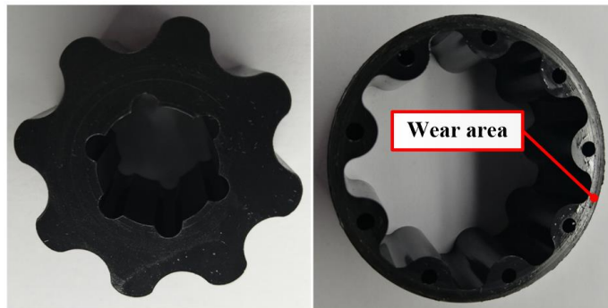
Fig. 19 The wear of PEEK inner and outer rotors after the test
