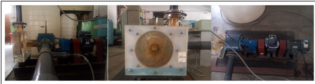
Figure 5. Closed pump test stand.
