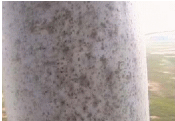
Fig. 1 Photograph of the leading edge with pitting erosion. A photograph from the company of wind turbine equipment maintenance [21].
