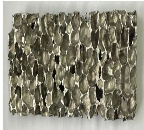
Fig. 1 Macro photograph of cell foam aluminum before laser forming
