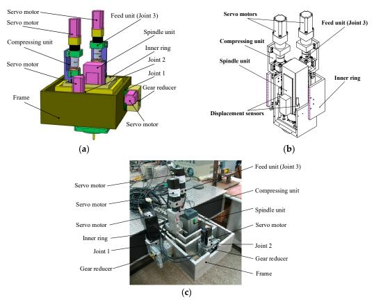
**Figure 1.** Structure and prototype of the designed end-effector: (a) the diagram of the end-effector structure; (b) the specific of the internal structure of the end-effector; and (c) the prototype of the end-effector.
