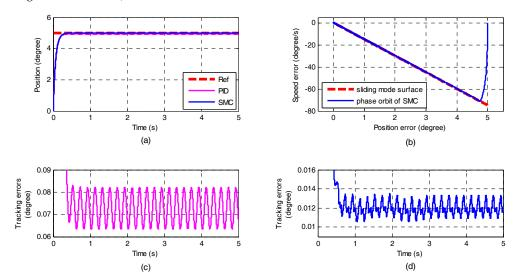
**Figure 5.** Simulation of step response of Joint 2: (a) Position tracking; (b) Phases trajectory diagram of SMC; (c) Tracking error of PID; and (d) Tracking error of SMC.
