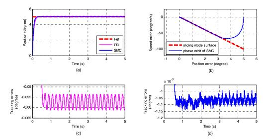
**Figure 4.** Simulation of step response of Joint 1: (a) Position tracking; (b) Phases trajectory diagram of SMC; (c) Tracking error of PID (proportional-integral-derivative); and (d) Tracking error of SMC (sliding mode controller).
