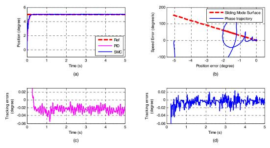
**Figure 10.** Experiment of step response of Joint 1: (a) Position tracking; (b) Phases trajectory diagram of SMC; (c) Tracking error of PID; and (d) Tracking error of SMC.
