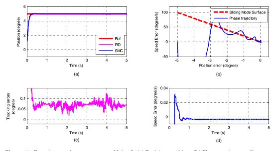
**Figure 11.** Experiment of step response of Joint 2: (a) Position tracking; (b) Phases trajectory diagram of SMC; (c) Tracking error of PID; and (d) Tracking error of SMC.
