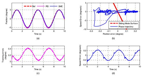
**Figure 13.** Experiment of sinusoidal response of Joint 2: (a) Position tracking; (b) Phases trajectory diagram of SMC; (c) Tracking error of PID; and (d) Tracking error of SMC.
