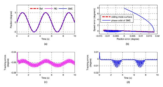
**Figure 6.** Simulation of sinusoidal response of Joint 1: (a) Position tracking; (b) Phases trajectory diagram of SMC; (c) Tracking error of PID; and (d) Tracking error of SMC.
