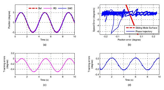
**Figure 12.** Experiment of sinusoidal response of Joint 1: (a) Position tracking; (b) Phases trajectory diagram of SMC; (c) Tracking error of PID; and (d) Tracking error of SMC.
