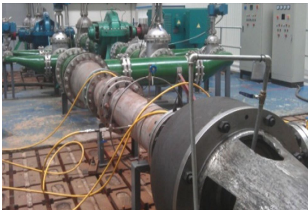
Fig. 5 Nuclear main pump model experiment system
