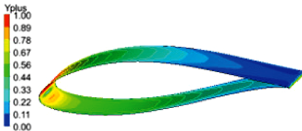
Fig. 4. (Color online) Grid wall y+ distribution.
