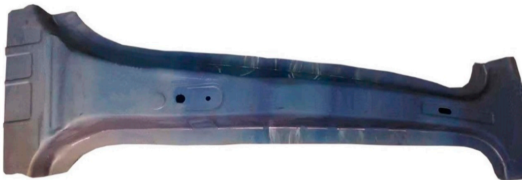
Figure 16. Hot stamping parts of the B-pillar.
