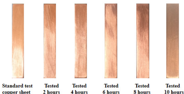
FIGURE 6. Corrosion test results of 68 # hydraulic oil.
