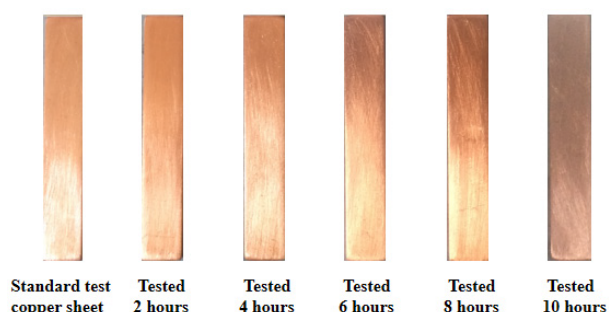
FIGURE 5. Corrosion test results of 46 # hydraulic oil.
