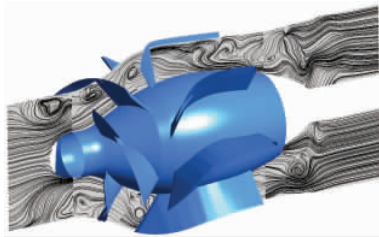
图 4 0.75Q_d 工况下子午面流线图 Fig. 4 Streamlines in meridional plane at 0.75Q_d condition
